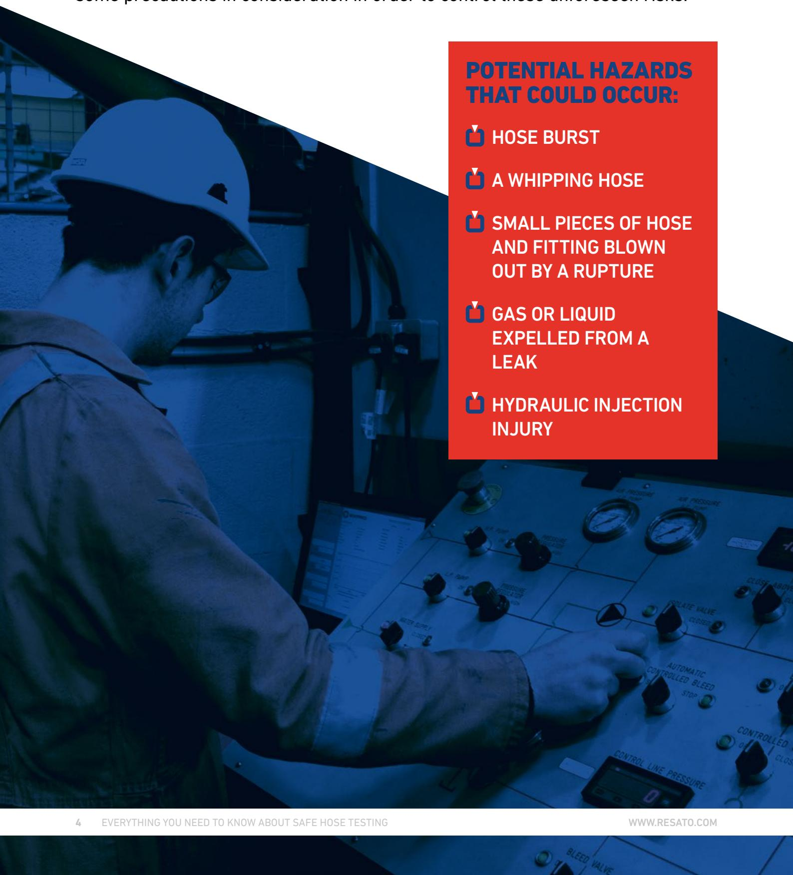
Resato hose testing benches are designed in such a manner that they can endure an unforeseen risk. The type of risk that could occur depends on the type of test. However, Resato designed its machines in such a manner that the operator is safe even in the worst-case scenario.
